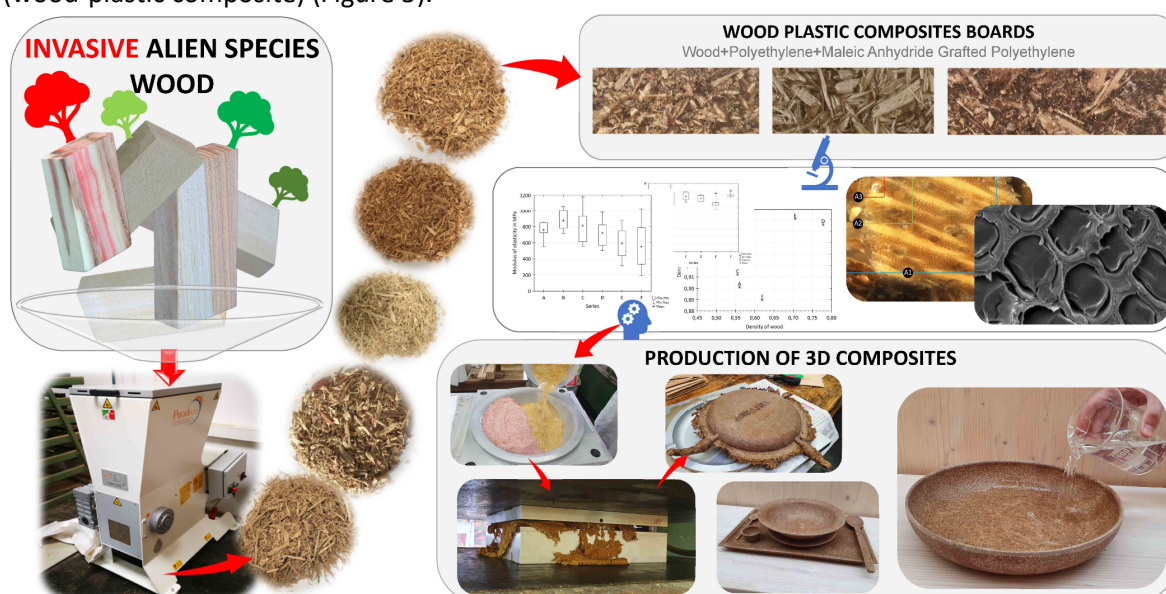
Fig. 4. WPC (wood-plastic composite) production from remains of invasive wood species processing.
